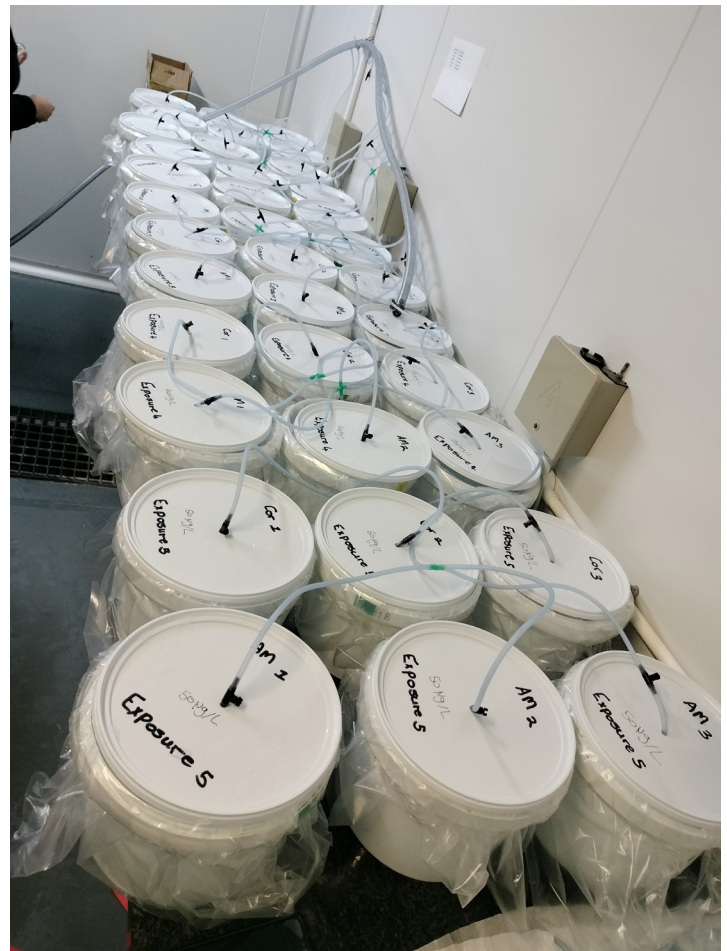
Laboratory setup exposing artificial mussels and the freshwater clam Corbicula sp. to a range of mercury concentrations.
