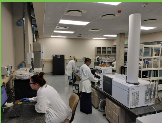
Laboratory 239 housing the LC-QTOF, GC- \mu ECD, F/GF-AAS and FIMS.
