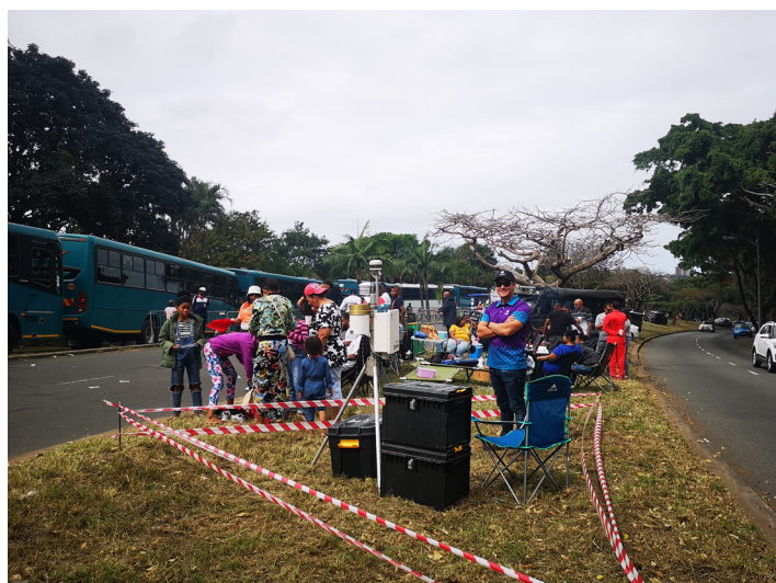
Tjaart Van Der Walt from the NWU team at one station along the route. The station consists of several instruments that measure weather conditions and air pollution.
